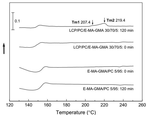
Fig. 4. The first DSC heating curves of the E-MA-GMA/PC (5/95) and LCP/PC/E-MA-GMA (30/70/5) blends with and without annealing at 200 °C.
