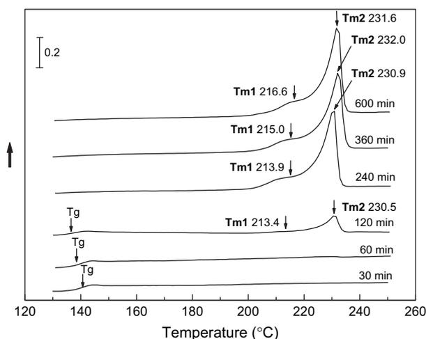
Fig. 3. The first DSC heating curves of the LCP/PC/E-MA-GMA (5/95/5) blend annealed at 200 °C for different times. The annealing time is marked above the corresponding curve.
