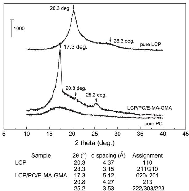
Fig. 2. The WAXD spectra of the pure PC, LCP and LCP/PC/E-MA-GMA (5/95/5) blend annealed at 200 °C for 10 h.
