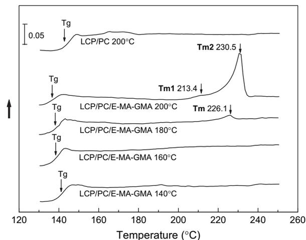
Fig. 1. The first heating DSC curves of the LCP/PC (5/95) and LCP/PC/E–MA–GMA (5/95/5) blends annealed at different temperatures for 2 h. The annealing temperature is marked under the corresponding curve.
